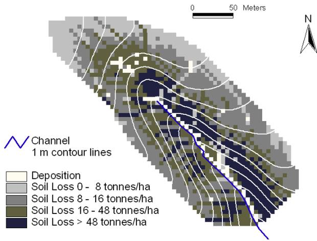
**Figure 3.** GeoWEPP-generated annual soil loss map for the Carpenter watershed, applying WEPP individual soil series parameters without the A horizon along with the bare soil management parameters.
