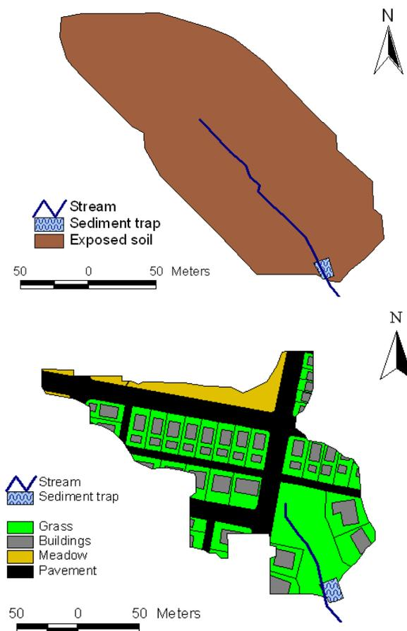
Figure 1. Management maps of the Carpenter watershed during (top) construction and (bottom) site stabilization. Watershed boundaries before and after construction were altered as a result of clearing and grading changes at the site.
