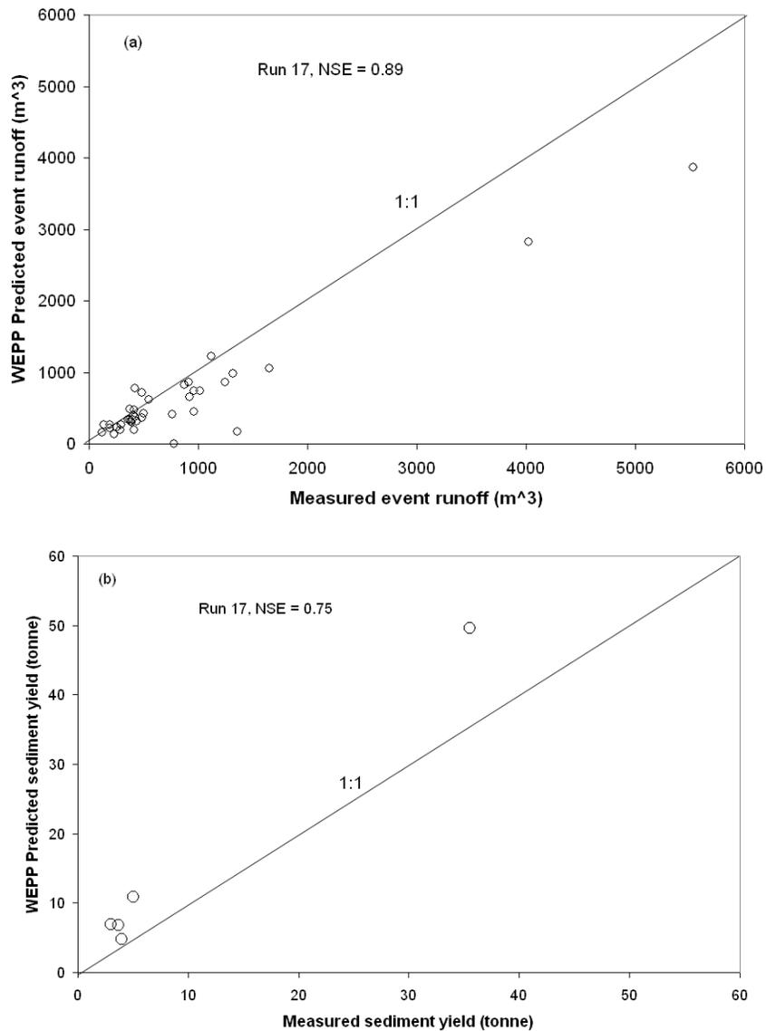
Figure 4. Observed and WEPP-predicted (a) runoff and (b) sediment yield for the Carpenter watershed for the post-construction phase ( $\tau = 10$  Pa).
