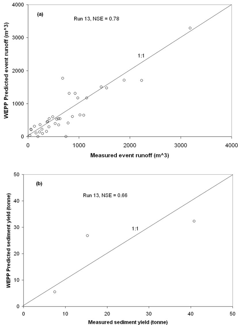
Figure 2. Observed and WEPP-predicted (a) runoff volumes and (b) sediment yields for the Carpenter watershed, applying WEPP soil parameter files for individual soil series without the A horizon along with the bare soil management parameters. The three data points in fig. 2b represent the three sediment depth survey events at the site.
