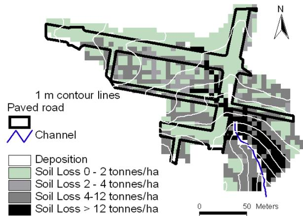
Figure 5. GeoWEPP generated annual soil loss map for the Carpenter watershed, applying optimal parameters for the post-construction phase.
