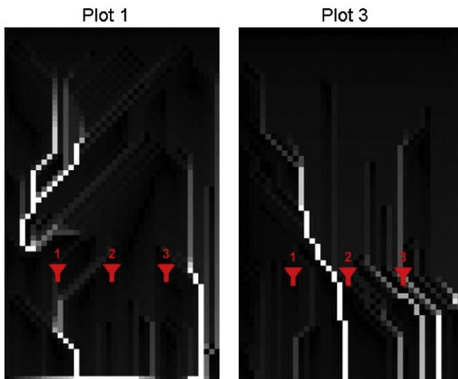
Fig. 6. Flow convergence zones and locations of miniflumes in vegetated plots 1 and 3; the lightest grid cells indicate areas where the accumulated flow was the highest.
