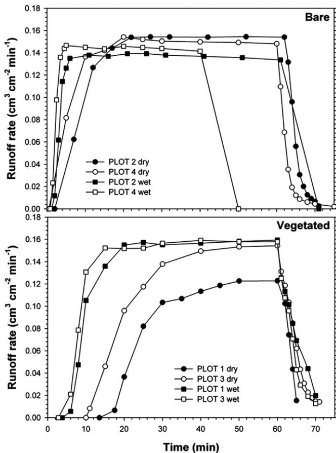
Fig. 2. Hydrographs of bare and vegetated plots under dry and wet conditions.
