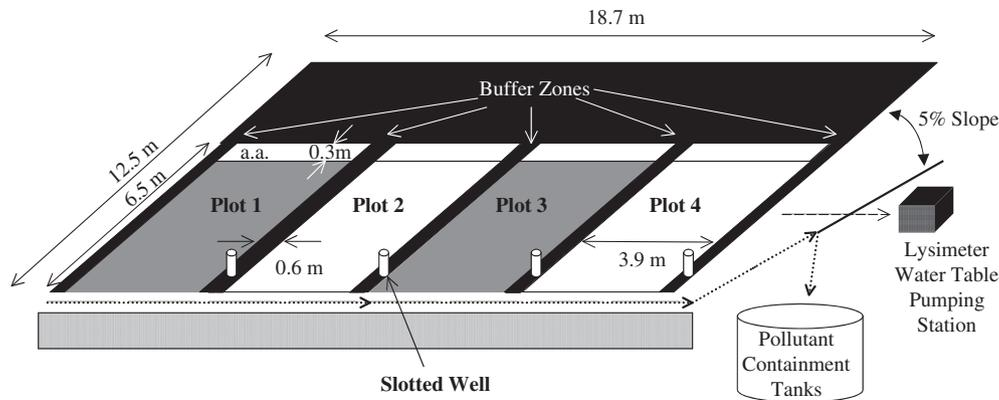
Fig. 1. Schematic diagram of lysimeter plots.
